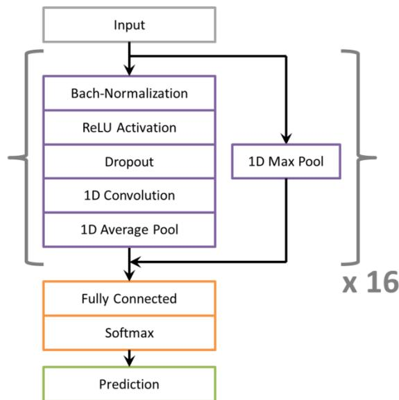
**Figure 2:** The proposed neural network architecture with repeated 16 1D convolutions with skip connections.
